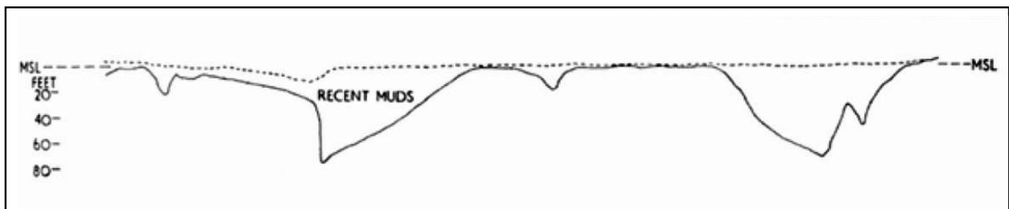
Fig. 6. East (left) to West (right) cross-section across Hobson Bay along the route of the former sewerage line. The solid line is the top of the Waitemata Sandstone and the pre-12000 years ago topography, whereas the dotted line is the present day surface of Holocene mud that now fills Hobson Bay. From Auckland Drainage Board in Searle (1959).
