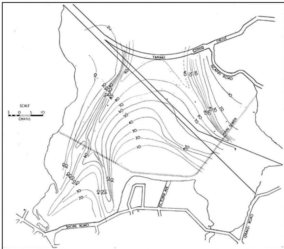
Fig. 5. Contour map of the Waitemata Sandstone–Holocene mud contact beneath Hobson Bay, which approximates the land surface contours prior to about 12000 years ago when sea level was 30 m or more lower. From Ministry of Works in Searle (1959). Contours in feet, scale in chains.
